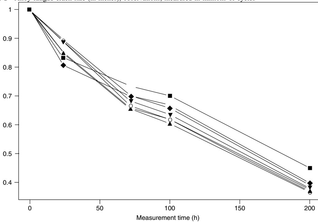
**Figure 2** Luminosity degradation in seven VFD devices
