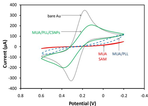
Figure 2. Cyclic voltammetry of 5 mM ferricyanide in aqueous 0.5 M KCl supporting electrolyte (100 mV/sec) at a bare gold electrode (black, dotted) and a gold electrode modified with a MUA SAM (red, solid), a MUA SAM and an adlayer of PLL (blue, dashed), and a MUA SAM with the PLL adlayer and a terminal layer of CSNPs (green, solid).
