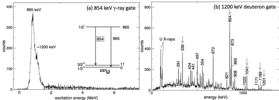
**Figure 5.** Spectra for  $^{237}\text{U}$ . (a) Deuterons in coincidence with the 854 keV  $\gamma$  ray. (b)  $\gamma$  rays in coincidence with the 1200 keV peak from (a).  $\gamma$  rays of interest are marked with arrows.
