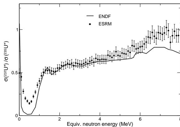
**Figure 3.**  $\sigma(^{236}\text{U}(n,f))/\sigma(^{234}\text{U}(n,f))$  ratios measured by the  $^{238}\text{U}(p,d)^{237}\text{U}/^{236}\text{U}(p,d)^{235}\text{U}$  surrogate measurement (data points) and compared to the literature value for the ratio (solid line).
