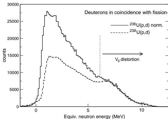
**Figure 2.** Comparison of deuteron spectra for the  $^{238}\text{U}(p,d)^{237}\text{U}$  and  $^{236}\text{U}(p,d)^{235}\text{U}$  reactions. The  $^{236}\text{U}(p,d)^{235}\text{U}$  data have been normalised to correct for the different integrated beam and target thicknesses in the two experiments. The region beyond  $\sim 6$  MeV is distorted as described in the text.
