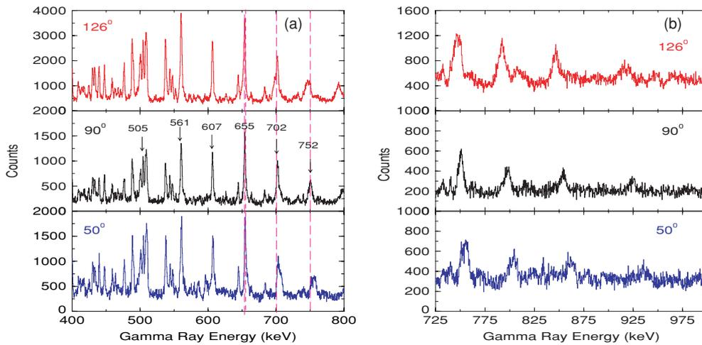
**Figure 1.** The Doppler shift of transitions in TSD1 observed at  $50^\circ$ ,  $90^\circ$  and  $126^\circ$  ( $122^\circ$  and  $130^\circ$  combined), respectively. The spectra (a) show the transitions from lower spin states and (b) show the transitions from higher spin states in TSD1.
