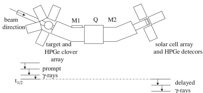
**Figure 1.** A typical set-up for a SASSYER experiment.
