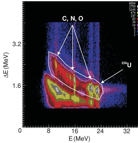
**Figure 1.** Particle identification  $\Delta E$ – $E$  spectrum for 24 MeV deuterons incident on a  $^{238}\text{U}$  target with counts plotted on a logarithmic scale. The spectrum was recorded by ring no 3 in the  $\Delta E$  detector, which is located at  $37.4^\circ$  with respect to the beam. The distribution inside the polygon corresponds to deuterons and the distribution below corresponds to protons.
