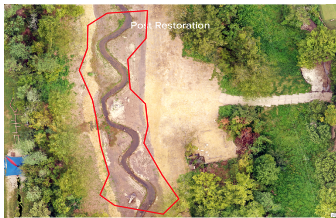
Image 3: Post- restoration drone imagery, georeferenced, and zoomed in for ease of comprehension within ArcMap.
