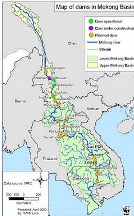
Figure 4: The Mekong River Basin and its associated dams in all stages of operation and planning
