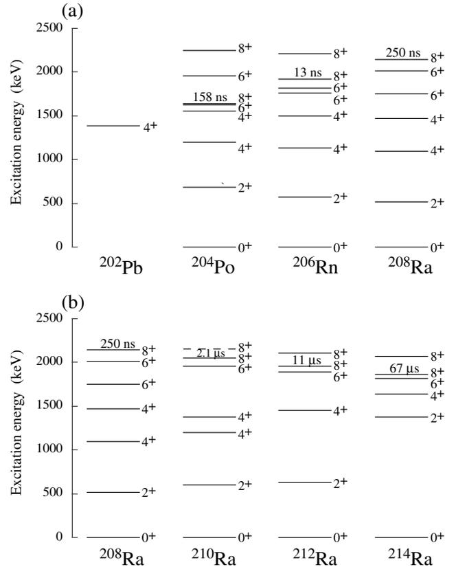
FIG. 5. Systematics of the (a)  $N = 120$  isotones and (b)  $Z = 88$  isotopes. Data are from Refs. [3–5,12,15,17] and this work. The second  $8^+$  state was not observed in  $^{210}\text{Ra}$  [5] but is proposed to lie at the energy shown.
