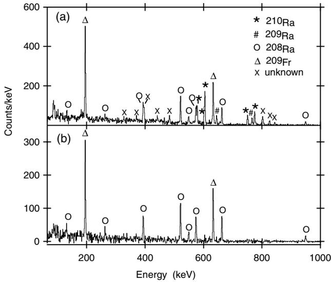
FIG. 1. (a) Delayed  $\gamma$  transitions observed within  $3 \mu\text{s}$  following a recoil implantation in the solar cell array. Most transitions may be assigned to  $^{210,209,208}\text{Ra}$  and  $^{209}\text{Fr}$  isotopes. (b) Time-subtracted isomer transitions; the spectrum of  $\gamma$ -ray energies detected within  $1\text{--}2.5 \mu\text{s}$  were subtracted from the spectrum collected within  $0\text{--}800$  ns after a recoil. Only short-lived species are observed.
