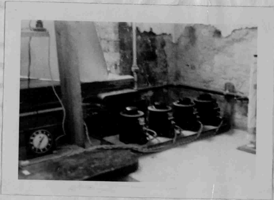
(a) The Voltage Transformers with an annealing oven for silica springs also shown.
