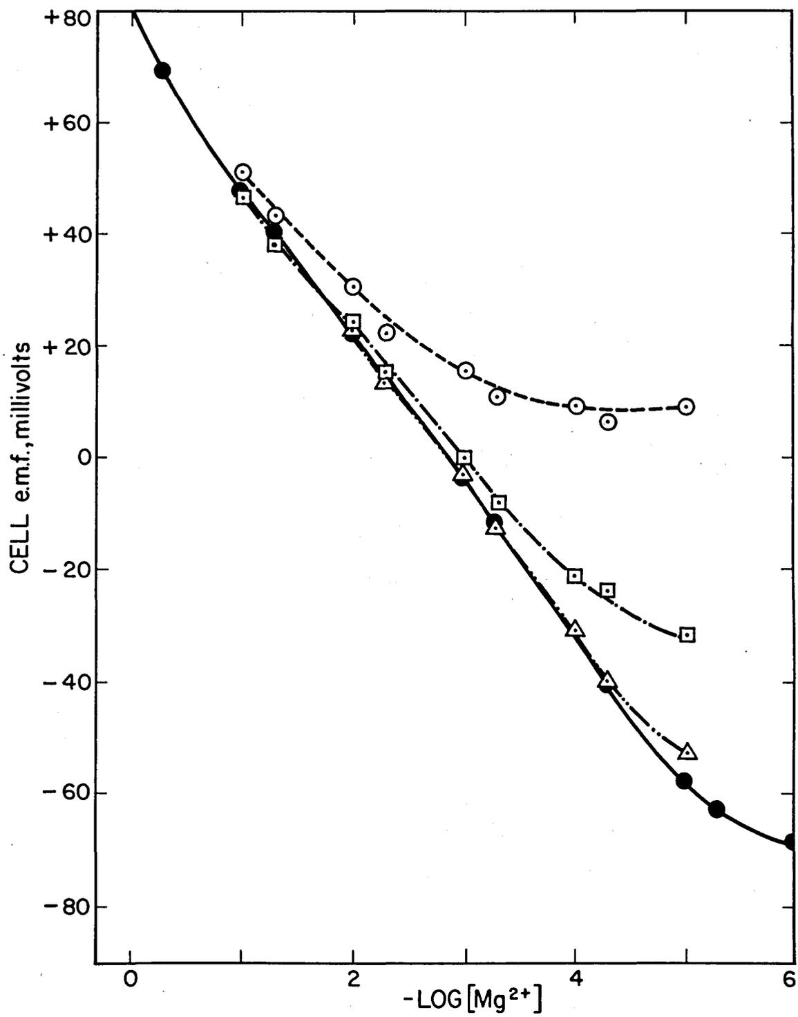
cation was held constant at either  $1 \times 10^{-1}$ ,  $1 \times 10^{-2}$ , or  $1 \times 10^{-3}$  M while the concentration of the divalent cation was varied from  $1 \times 10^{-1}$  to  $1 \times 10^{-5}$  M. The pH of the solutions was adjusted to  $7.0 \pm 0.1$  by the addition of small increments of either HCl or NaOH.
