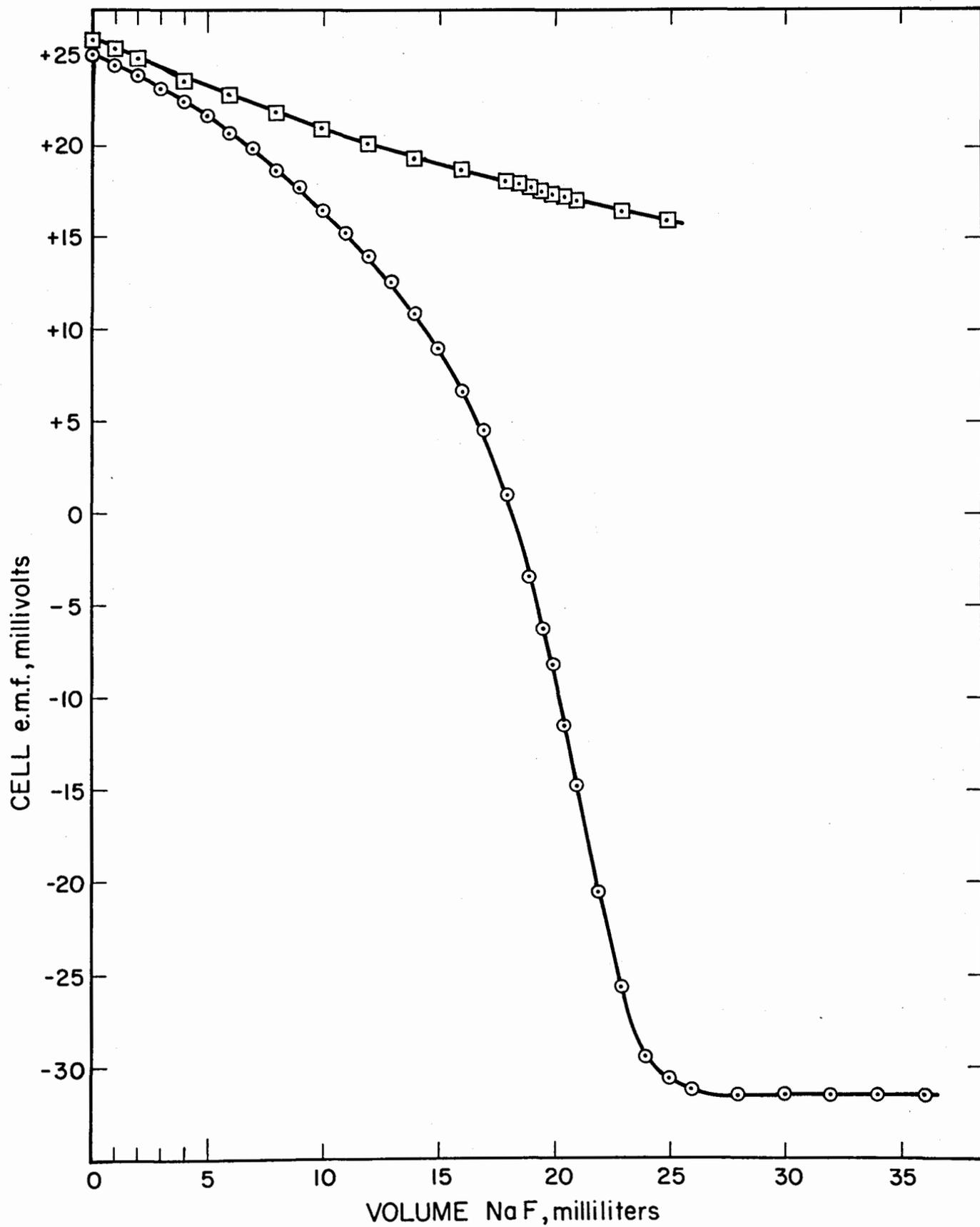
Since the concentration of fluoride ion was twice this value, the solubility product was  $(7.4 \times 10^{-4})(1.5 \times 10^{-3})^2$ , or  $1.7 \times 10^{-9}$ . A similar calculation from the data of the magnesium titration with an equivalence point potential of +17.8 mv gave  $2.0 \times 10^{-6}$  as the solubility product of magnesium fluoride.
