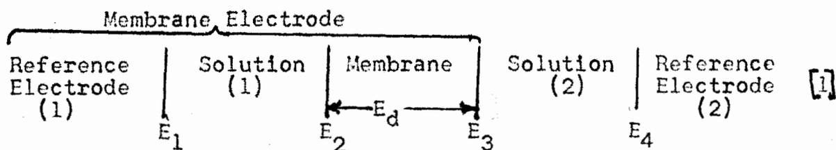
The emf of this cell is the sum of the phase-boundary potentials  $E_1$ ,  $E_2$ ,  $E_3$ , and  $E_4$  and a diffusion potential  $E_d$  within the membrane:
