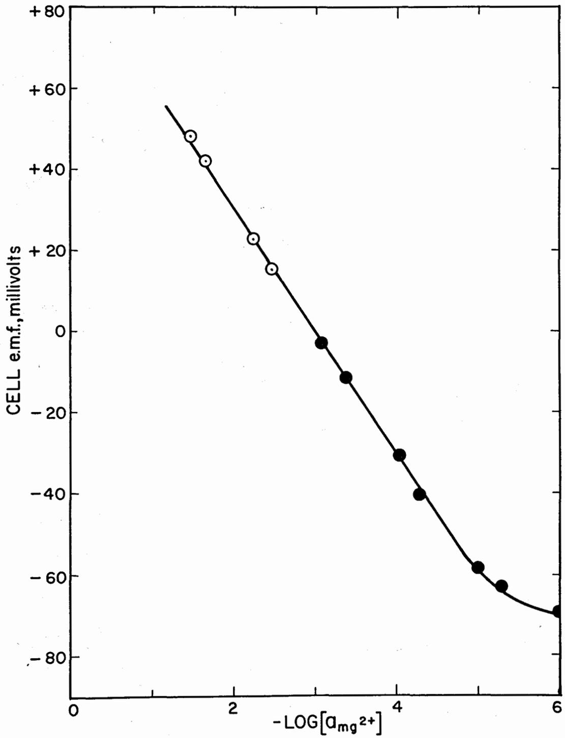
coefficient  $r = 0.9998$ ). The experimentally obtained slopes of  $30.0 \text{ mv}/p_a\text{Ca}^{2+}$  and  $30.1 \text{ mv}/p_a\text{Mg}^{2+}$  were in good agreement with the theoretical slope of  $30.1 \text{ mv}/p_a\text{M}^{2+}$  predicted by the Nernst equation. No anion effect on the activity response of the electrode was observed. Once ionic concentrations have been converted to activities, a straight line plot is obtained regardless of the anion associated with the metal cation.
