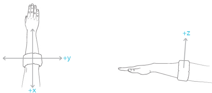
Figure 4: A representation of the Myo coordinate system for accelerometer and gyroscope [5].
