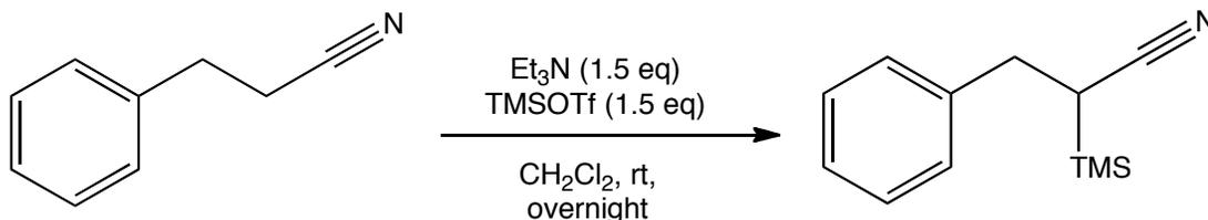
**Figure 15.** Silylation of 3-phenylpropionitrile
