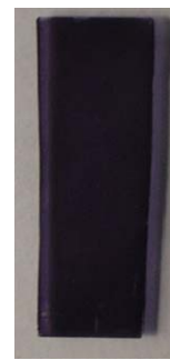
Figure 5: (left) Film growth comparisons of 1L(PLL) , 3L (PLL/PSS/PLL), and 5L (PLL/PSS/PLL/PSS/PLL) multilayer-polymer multilayer-nanoparticle films. (right) Actual image of 5L multilayer-polymer multilayer-nanoparticle film system on a glass slide. [From ref. 22]
