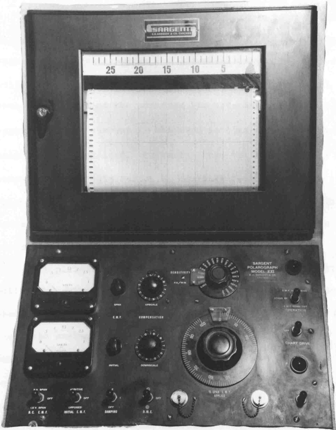
Figure 6. The Sargent-Heyrovsky Model XXI Polarograph
