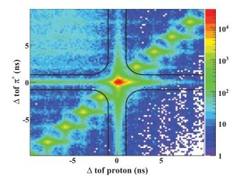
FIG. 2. (Color online)  $\Delta tof_{\pi^+}(ns)$  versus  $\Delta tof_p(ns)$ : Particle identification cut for a sample of events that pass a 10% confidence level cut when kinematically fit to the hypothesis  $\gamma p \to p \pi^+ \pi^-(\pi^0)$ . The black lines indicate the timing cuts. Note the logarithmic scale on the intensity axis.
