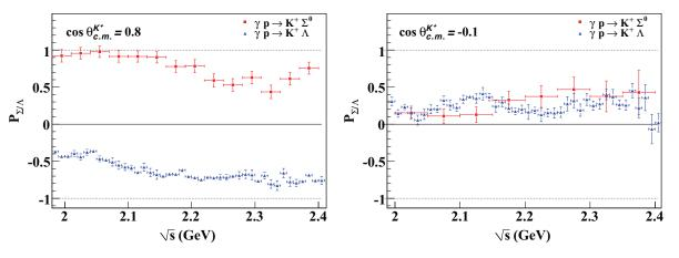
FIG. 17. (Color online) The SU(6) prediction of  $P_{\Sigma} \approx -P_{\Lambda}$  is seen to hold at (a) forward angles, but is broken for certain (b) mid- and backward-angle kinematics. The  $P_{\Lambda}$  values are taken from Ref. [25].
