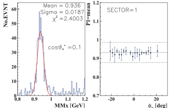
FIG. 8. (Color online) An example of a neutron missing mass fit for sector 1 by a single Gaussian function in the bin at  $\cos \theta_\pi = 0.1$ ,  $W = 1.11 \text{ GeV}$ , and  $Q^2 = 2.44 \text{ GeV}^2$  (left), and the neutron missing mass  $\phi_\pi$  dependence for sector 1 (right). Dashed lines are defined in the text.
