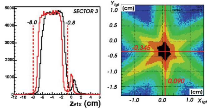
FIG. 4. (Color online)  $z$ -vertex distribution for sector 3 before (black solid line) and after (red solid line) vertex correction (left). The vertex cuts are illustrated by the vertical dashed lines. Reconstructed  $X$  and  $Y$  target positions, showing an offset of  $X_{\text{tgt}} = 0.90$  mm and  $Y_{\text{tgt}} = -3.45$  mm, respectively (right).
