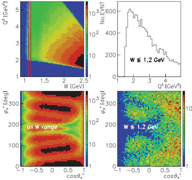
FIG. 9. (Color online) Examples of Monte Carlo simulation results:  $Q^2$  versus  $W$  and the angular distribution  $\phi_\pi^*$  versus  $\cos\theta_\pi^*$  for all  $W$  (left column) and yield versus  $Q^2$  and the angles  $\phi_\pi^*$  versus  $\cos\theta_\pi^*$  for  $W \leq 1.2$  GeV (right column) as a snapshot after GSIM reconstruction but still without the GPP step. The two vertical solid lines on the top-left plot show the  $W$  region between 1.10 and 1.16 GeV of interest.
