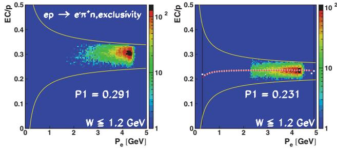
FIG. 3. (Color online) Optimized sampling fraction constant of EC versus electron momentum with  $W \leq 1.2$  GeV for the experimental data (left) and Monte Carlo simulation (right). The solid lines (left) show the  $\pm 3\sigma$  cuts from all electron fit.  $P1$  is the sampling fraction from fit.
