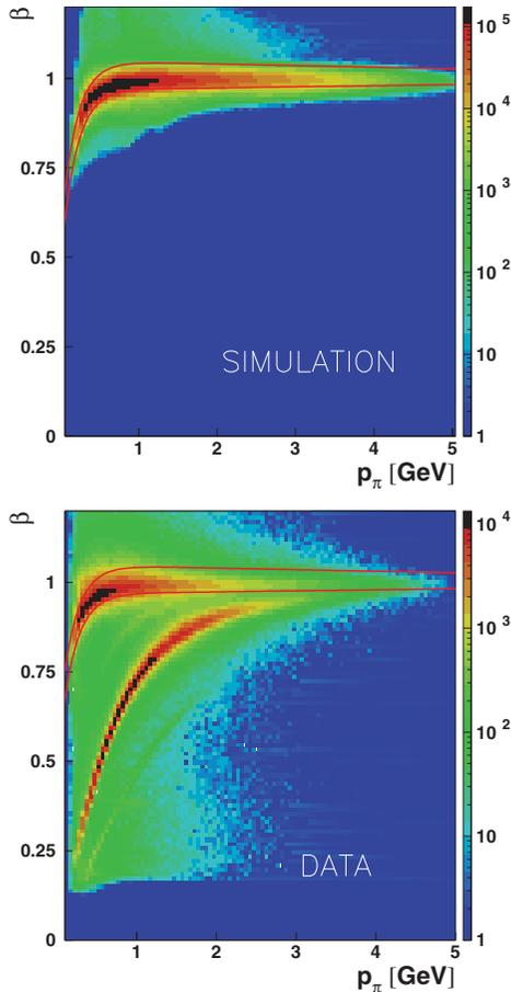
FIG. 5. (Color online) The particle velocity distribution  $\beta$  versus particle momentum. The pion velocity sample is fit by a function of the form  $A + \exp(B + Cp_\pi)$  to generate the  $\beta$  cut for both simulation (upper) and experimental data (lower).
