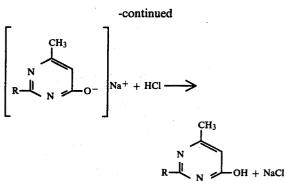
Recently the above conventional manufacturing process has been improved and optimized by a continuous ring-closure/neutralization process as claimed in U.S. Pat. No. 4,014,879, issued Mar. 29, 1977.
