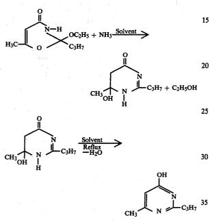
It is the removal of the water from the intermediate between the oxazinone and the pyrimidine which pro-4۵ vides the superior product of the present invention.
