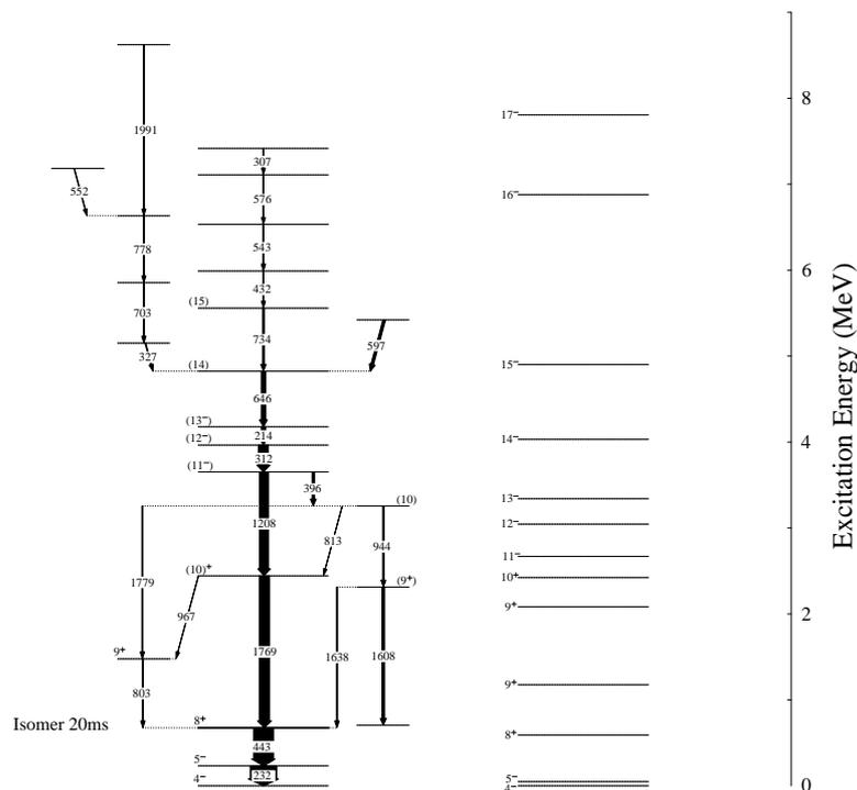
Figure 3: Preliminary results (left) Level scheme with previously unobserved levels (right) Calculated level scheme (NuShell [14]) with levels corresponding to observed levels shown.
