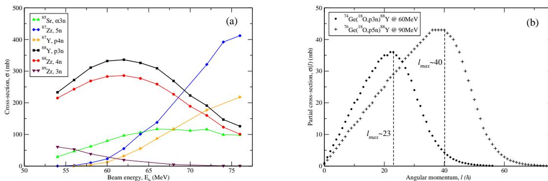
Figure 1: PACE4 [1, 2] calculations (a) Cross-section calculations for  $^{74}\text{Ge}(^{18}\text{O},\text{p}3\text{n})^{88}\text{Y}$  (b) Partial cross-sections for  $^{74}\text{Ge}(^{18}\text{O},\text{p}3\text{n})^{88}\text{Y}$  and  $^{76}\text{Ge}(^{18}\text{O},\text{p}5\text{n})^{88}\text{Y}$
