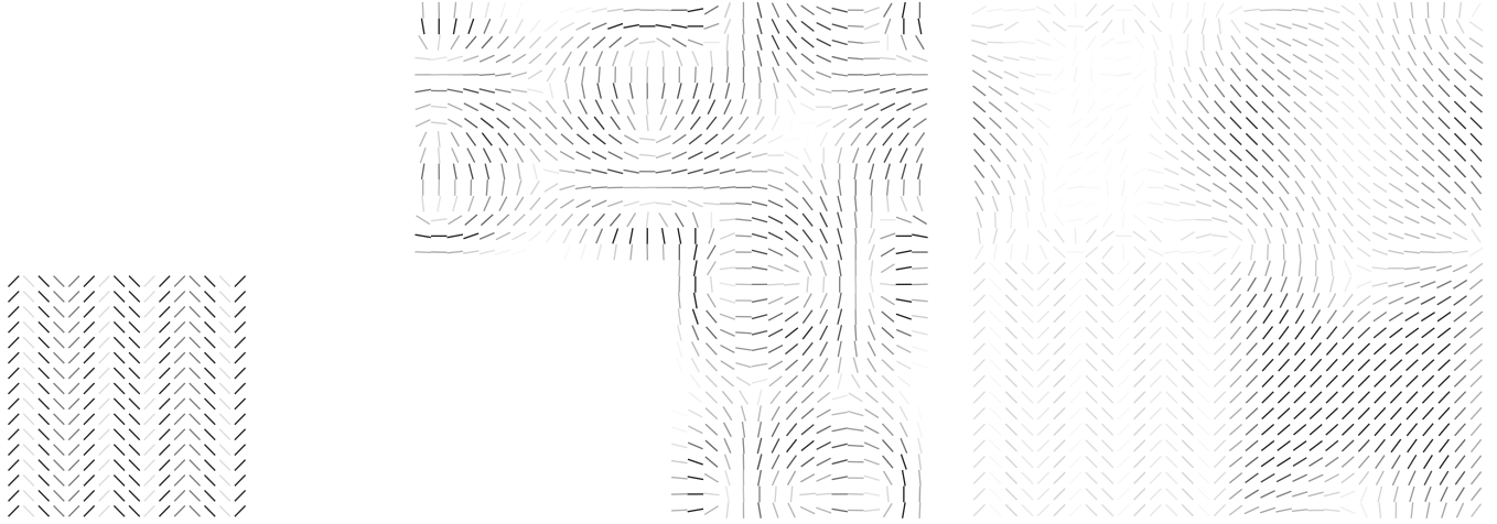
FIG. 2. Numerical instability in extending maps. The original map (left panel) is a single B -type Fourier mode. It was extended using the mean-field method, with results shown in the center and right panels. The center panel shows the result of the extension when the Gaussian random process had no B power. The result is an attempt to match the input B mode using only E modes, leading to numerical instability: the maximum polarization level in the extended region is 590 times that of the original map, so that the original map (lower left quadrant) is invisible. The right panel shows the result obtained when P_B is taken to be 0.01P_E . In this case, the peak polarization level is 4.3 times that in the extended region.
